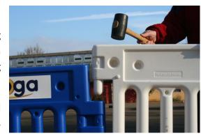
next, again with a push fit system, keep fingers clear of the push fit joint. If the joints are tight, use a rubber mallet to persuade the panel into place.
